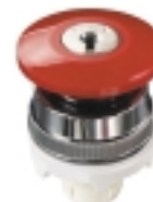
Push Key Push Button. Manual push "In". Spring return. Turn key counter- clockwise to lock "Out"; clockwise to unlock. Key withdrawable locked or unlocked. Black only.
